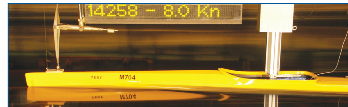
Testing of water resistances in test canal
